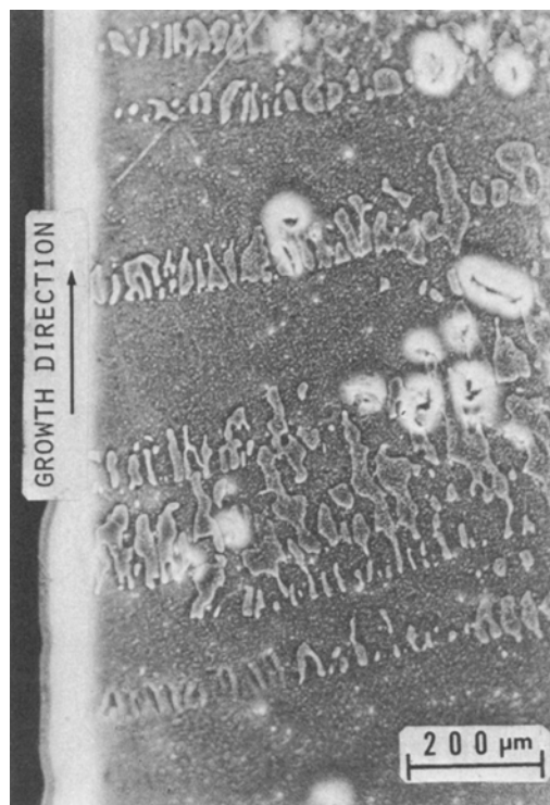
Figure 6 Typical occurrence of foreign phase precipitates and voids in a grown crystal (negative phase contrast).
